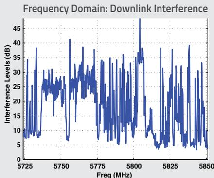
Maximum Interference Level at Receiver above the Noise Floor in a typical 1 second period
