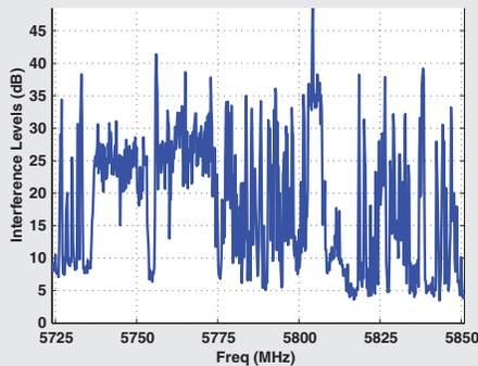
Maximum Interference Level at Receiver above the Noise Floor in a typical 1 second period
