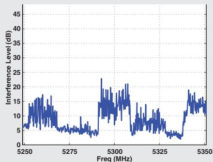
Maximum Interference Level at Receiver above the Noise Floor in a typical 1 second period
